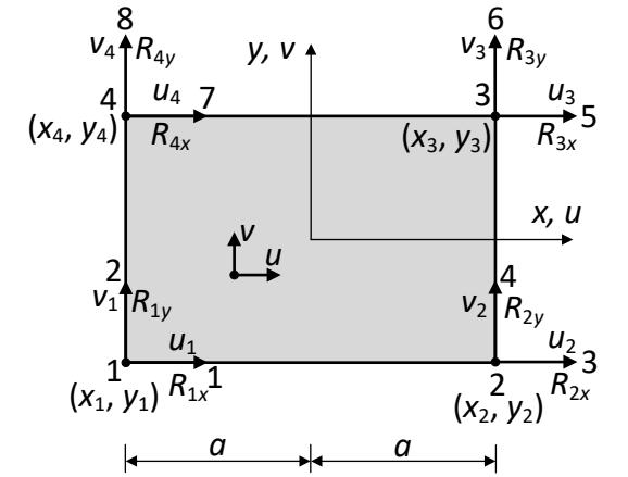
$$\mathbf{C} = \begin{bmatrix} 1 & -a & -b & ab & 0 & 0 & 0 & 0 \\ 0 & 0 & 0 & 0 & 1 & -a & -b & 0 \\ 1 & a & -b & -ab & 0 & 0 & 0 & 0 \\ 0 & 0 & 0 & 0 & 1 & a & -b & -ab \\ 1 & a & b & ab & 0 & 0 & 0 & 0 \\ 0 & 0 & 0 & 0 & 1 & a & b & ab \\ 1 & -a & b & -ab & 0 & 0 & 0 & 0 \\ 0 & 0 & 0 & 0 & 1 & -a & b & -ab \end{bmatrix}$$
