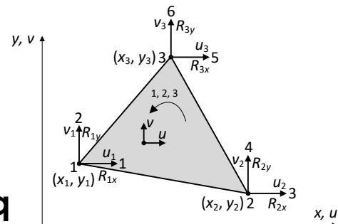
$$\mathbf{Q} = \begin{Bmatrix} \mathbf{Q}_1 \\ \mathbf{Q}_2 \\ \mathbf{Q}_3 \end{Bmatrix} = \begin{Bmatrix} Q_{1x} \\ Q_{1y} \\ Q_{2x} \\ Q_{2y} \\ Q_{3x} \\ Q_{3y} \end{Bmatrix} = \begin{Bmatrix} Q_1 \\ Q_2 \\ Q_3 \\ Q_4 \\ Q_5 \\ Q_6 \end{Bmatrix} = \int_A \mathbf{N}^T \mathbf{q} h dA = \int_A \begin{bmatrix} N_1 & 0 \\ 0 & N_1 \\ N_2 & 0 \\ 0 & N_2 \\ N_3 & 0 \\ 0 & N_3 \end{bmatrix} \begin{Bmatrix} q_x \\ q_y \end{Bmatrix} h dA$$
