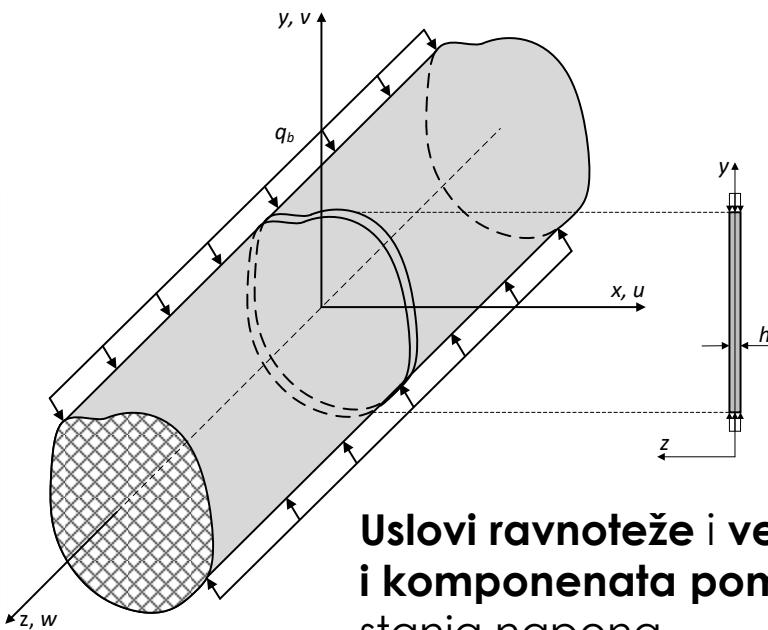
$$\boldsymbol{\sigma}^T = \{\sigma_x \neq 0 \quad \sigma_y \neq 0 \quad \sigma_z \neq 0 \quad \tau_{xy} \neq 0 \quad \tau_{yz} = 0 \quad \tau_{zx} = 0\}$$
