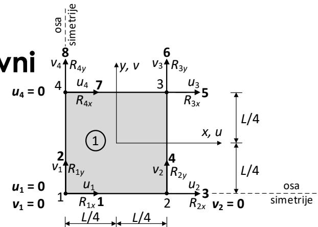
$$\mathbf{u} = \mathbf{N}\mathbf{d} \rightarrow \begin{Bmatrix} u(x,y) \\ v(x,y) \end{Bmatrix}^{(1)} = \mathbf{N}^{(1)}\mathbf{d}^{(1)} = \begin{Bmatrix} 0,000250 + 0,00050x \\ -0,000075 - 0,00015y \end{Bmatrix} \text{ m}$$
