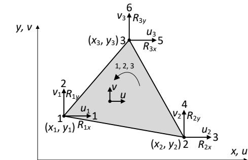
$$\mathbf{d} = \mathbf{C}\boldsymbol{\alpha} \rightarrow \begin{Bmatrix} d_1 \\ d_2 \\ d_3 \\ d_4 \\ d_5 \\ d_6 \end{Bmatrix} = \begin{Bmatrix} u_1 \\ v_1 \\ u_2 \\ v_2 \\ u_3 \\ v_3 \end{Bmatrix} = \begin{bmatrix} 1 & x_1 & y_1 & 0 & 0 & 0 \\ 0 & 0 & 0 & 1 & x_1 & y_1 \\ 1 & x_2 & y_2 & 0 & 0 & 0 \\ 0 & 0 & 0 & 1 & x_2 & y_2 \\ 1 & x_3 & y_3 & 0 & 0 & 0 \\ 0 & 0 & 0 & 1 & x_3 & y_3 \end{bmatrix} \begin{Bmatrix} \alpha_1 \\ \alpha_2 \\ \alpha_3 \\ \alpha_4 \\ \alpha_5 \\ \alpha_6 \end{Bmatrix}$$
